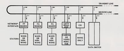
\* FF = FIXED FREQUENCY (DEDICATED CHANNELS) FA = FREQUENCY AGILE (SWITCHED CHANNELS) CIU = CABLE INTERFACE UNIT (WANGBAND)
